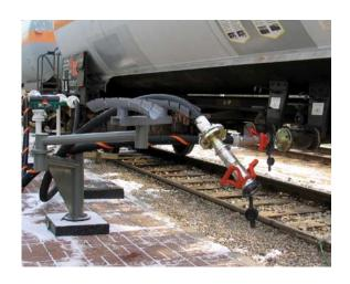
Just like their TODO-MATIC® stable mates, TODO-GAS® couplings remove the human error element from LPG transfer operations by ensuring that the valves are closed before disconnection is possible.
