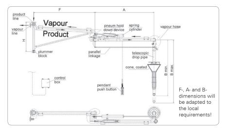
The E2630 is the most economical solution for the loading process with vapor return. Reliable and easy handling is given by small weight and little offset. An E2630 may also be used where the available space is limited, e. g. existing loading stations with low roof heights.
