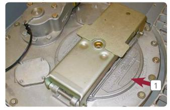
1 Emergency Venting at a massive 7000m<sup>3</sup>/hr via the pressure actuated fill cap safeguards against tank explosion in the event of a fire.
