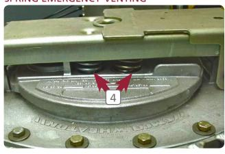
Four visible, corrosion proof, plated spring emergency venting. The springs are not shrouded in a rubber sleeve, which was the cause of a major failure on another manufacturer's manhole cover due to rainwater ingress that could not dry out and consequently corroded the single spring. The corrosion was not evident, as the spring was not visible. The UK Health & Safety Commission identified this as a cause of failure in an official report.
